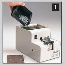
Load screws into the hopper. There is no side to load unit and no gates to limit capacity.
