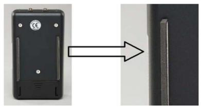
The rails on the RT-500 are made of conductive rubber. Soft rubber rails provide the highest level of surface contact for greater accuracy.
