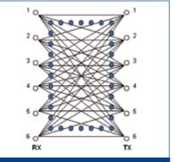
Scan mode 3-4: low speed / high resolution Minimum object detection Flat = 0.2 (thickness) x 75 (width) mm Cylindrical objects = Ø 6 mm
