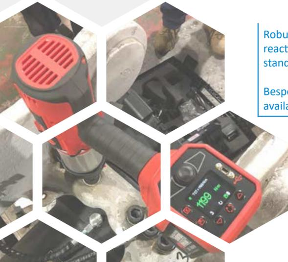
The square drive is quickly and easily replaceable
