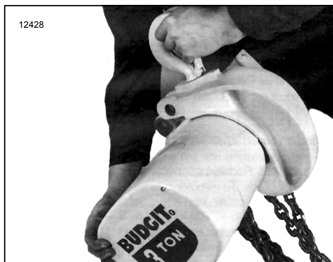
Figure 7-2. Removing 3 Ton Hanger Bracket from Hoist Frame
