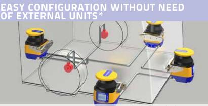
Up to 4 LASER SENTINEL can be easily connected to each other through Ethernet-based safe communication bus. Only one of them, the Master, receives power, has inputs and outputs onboard and keeps the memory of the configuration of the entire system. The other scanners, the Slaves, are connected to the Master with a single cable that also give them power. The syncronization of the four scanners is an integrated function: there is no need of external control units.
