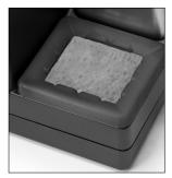
The least harmful cleaning method. Keep the sponge damp with distilled water when working to avoid tip wear.
