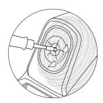
If the tip is very dirty, JBC first recommends cleaning it with the wiper to remove excess solder.
