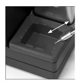
Wiping: Use the slots to remove remaining particles.
