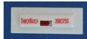
BAD Indicator (excessive shock, DO NOT install!)
