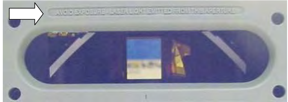
Warning on AXIOM Laser Exit Window to Avoid Exposure
