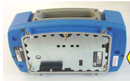
AXIOM Scan Head Shock Indicator Location
