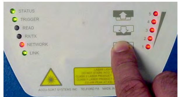
AXIOM Button and LEDs involved with Laser Shutoff
