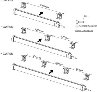
■ Installation Procedure (use Holding bracket\*) Install the holding bracket in the main unit, install on a sturdy surface with
