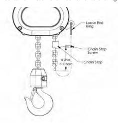
Figure 12. Attaching Loose End of Chain
