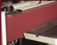
The JET<sup>®</sup> Oscillating Edge Sander showcases a unique oscillating feature. Oscillation of the belt means the sandpaper never runs a true straight line, which allows the unit to sand with more of the usable sandpaper and eliminates sanding lines. With a large sanding surface, you can process both the edge and surface of many different board sizes. Contour sanding is also an option when using the large built-in table around the drum over the motor.
