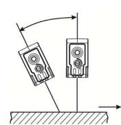
In the presence of moving backgrounds like conveyor belts, especially having a dark or shiny surface, the best object detection performance can be obtained by mounting the sensor at an angle (max 30°) with respect to the horizontal plane, as shown in the figure
