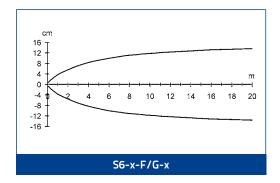
The detection diagrams indicate the typical operating distance with excess gain 1.
