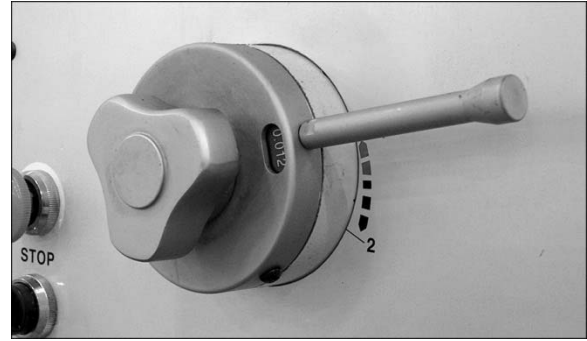
Figure 13: Feed rate setting mechanism
