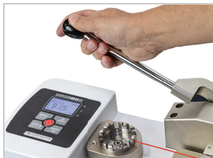
▲ An ergonomic lever easily applies force and releases the sample.
