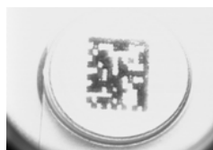
Washed out and Axial Distortion
