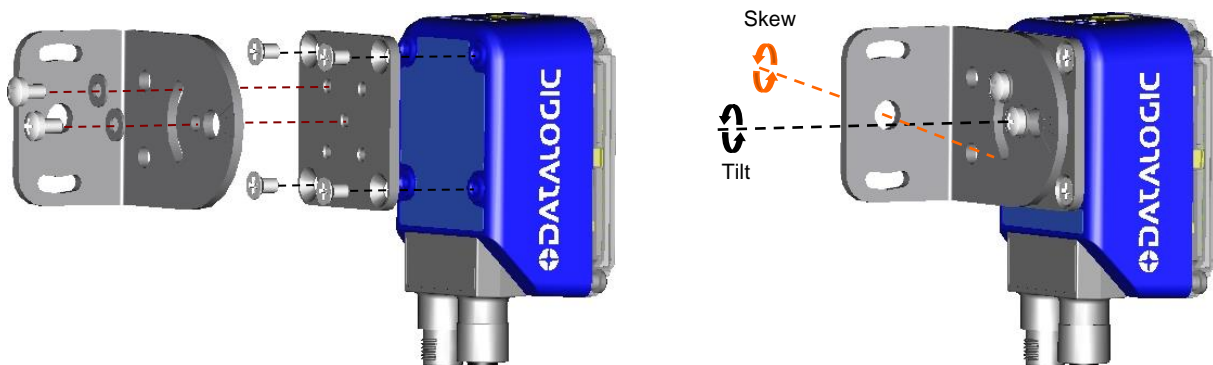
Figure 2 – Positioning with Mounting Bracket
