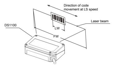
Figure 21 - "Picket-Fence" Scanning Mode
