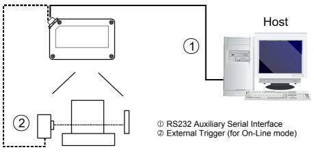
Figure 17 – Point-to-Point Layout
