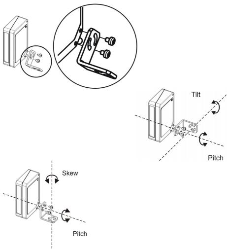
Figure 3 - Positioning with Mounting Bracket
