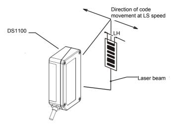
Figure 20 - "Step-Ladder" Scanning Mode
