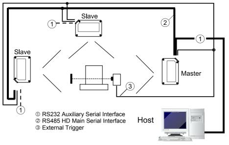
The main and auxiliary ports are connected as shown in the following figure.
