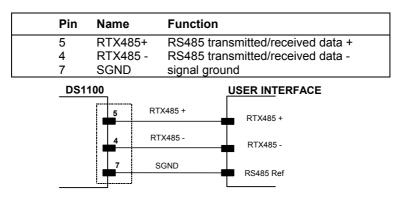
Figure 7 - RS485 Half-Duplex Connections
