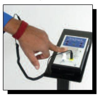
Attach wrist strap, step on duel plate and press metal button
