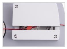
As the test begins, serrated cams engage the sample. A pinch guard (red tab shown above) automatically rotates into position, for added safety.
