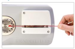
The tester automatically starts when the sample is loaded, and returns to home when the sample breaks. Adjustable terminal fixture accommodates wire diameters up to 0.25 in (6.3 mm)
