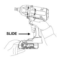
2. To remove the battery pack, press the button on the top of the battery pack and release the battery.
