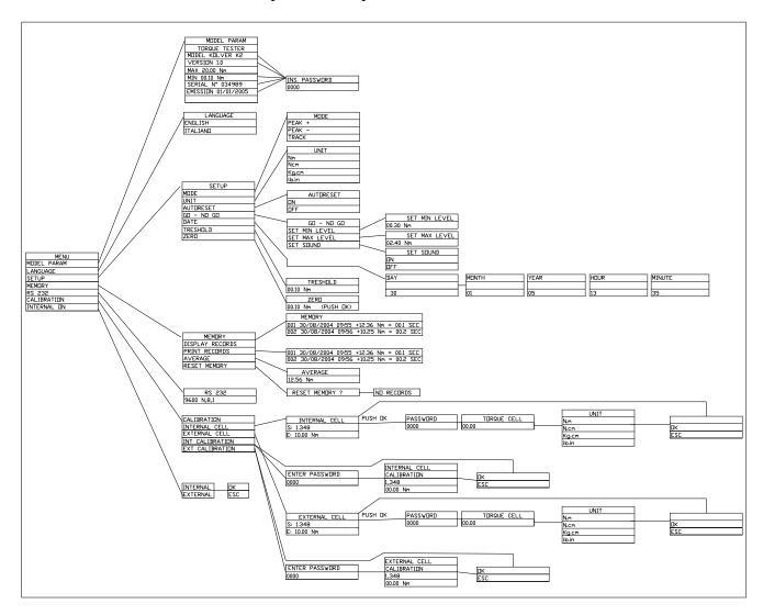
Push  $^{\wedge}$  key to enter the menu from the main screen. To move through the menus push  $^{\wedge}$  or  $\vee$  keys. The indicator < on the right side of the screen will signal the selected option. Push "OK" key to confirm the desired option.
