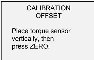
4. Place the torque sensor vertically in a fixture free from vibration, then press **ZERO**. The gauge will calculate offsets, and the display appears as follows:
