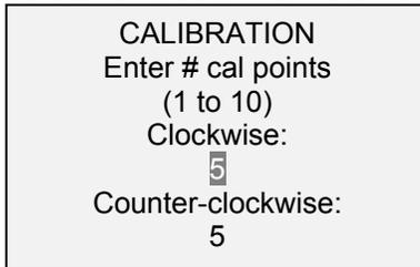
The sensor can be calibrated at up to 10 points in each direction. Enter the number of calibration points for each direction. At least one point must be selected for each direction.
