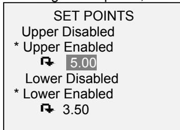
Either one, two, or none of the set points may be enabled. To toggle between the clockwise and counter-clockwise directions, press the **DIRECTION** key.
