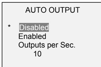
Select **Enabled** to activate automatic output. The number of outputs per second can be set to 1, 2, 5, 10, 25, 50, 125, or 250. The capabilities of the receiving device should be considered when selecting the data output rate.
