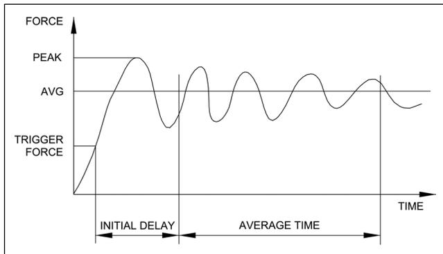
Average mode is used to obtain an average force reading over a specified period of time. This reading also represents the kinetic coefficient of friction for the M5-2-COF gauge. Applications include measurement of peel force, COF, muscle strength, frictional force, and other tests requiring time-averaged readings.
