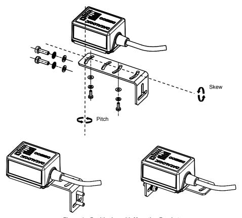
Figure 4 – Positioning with Mounting Bracket
