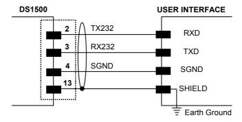
Figure 7 - RS232 Main Interface Connections
