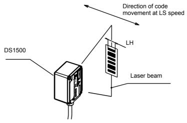
Figure 24 - "Step-Ladder" Scanning Mode
