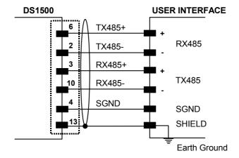
Figure 8 - RS485 Full-duplex Connections
