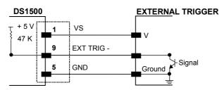
Figure 13 - External Trigger Input Command using Scanner Power
