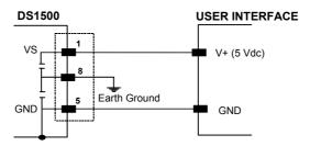
Figure 6 - Power Supply Connections
