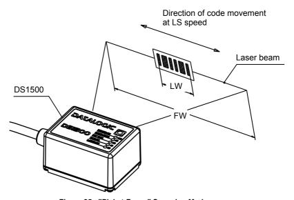
Figure 25 - "Picket-Fence" Scanning Mode
