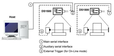
Figure 21 - Pass-Through Layout
