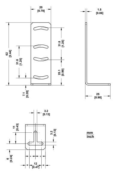
Figure 3 – Mounting Bracket Overall Dimensions
