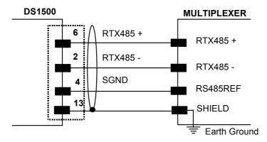
Figure 10 - RS485 Half-duplex Connections
