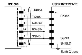
Figure 9 - RS485 Full-duplex Connections Using Only TX Signals
