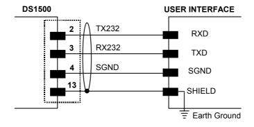
Figure 12 - RS232 Auxiliary Interface Connections
