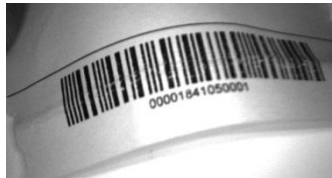
Figure 23 - Barcode Printed on Curved Surface Readable by Matrix 410N in spite of Image Optical Distortion
