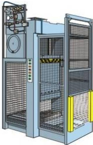
The safety device must protect the operator from being squashed between the top and bottom parts or the machined part during the fast approach phase.
