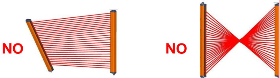
**Fig. 14 – Light curtains orientation**
