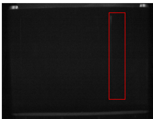
Cross-Belt FOV Image (note seam)
