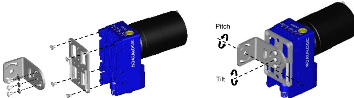
Figure 4 –Positioning with Body Mounting Bracket (Back)
