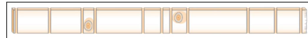
Dynamic Optimization™ for material yield & defect optimization. Get high quality parts from lower grades of lumber.
