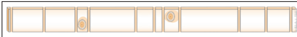
Dynamic Optimization™ for material yield & defect optimization. Get high quality parts from lower grades of lumber.
