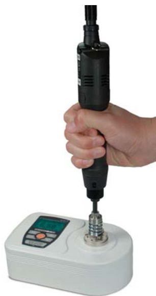
Fig. 2 Proper use of a rundown fixture with an electric torque tool. Note the axial vertical alignment.
