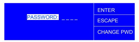
Push the MENU button for 5 secs. Push the encoder knob and enter the four numbers of the password (default password is: 1111). Once entered the password, turn the encoder to **ENTER**, push it and the unit will show the first screen.
