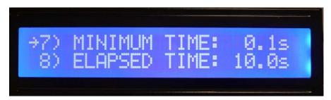
8) **ELAPSED TIME:** This is the maximum time that the tool will run. The tool stops running when this time is met.
