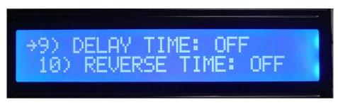
**10) REVERSE TIME**: This option will automatically start a reverse cycle after a torque reached signal or a time out signal (see also point 4 and 5). You can select a time between OFF (function excluded) and up to 10 seconds. During the reverse cycle, it is necessary to keep the lever pressed or the start signal otherwise the screwdriver will stop before the pre-set time.
