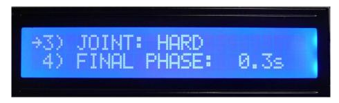
**IMPORTANT:** An incorrect selection of the joint type can result in inaccurate torque output.
