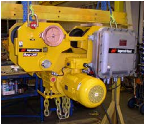
Electric Chain Hoists For Explosion Proof Environments
